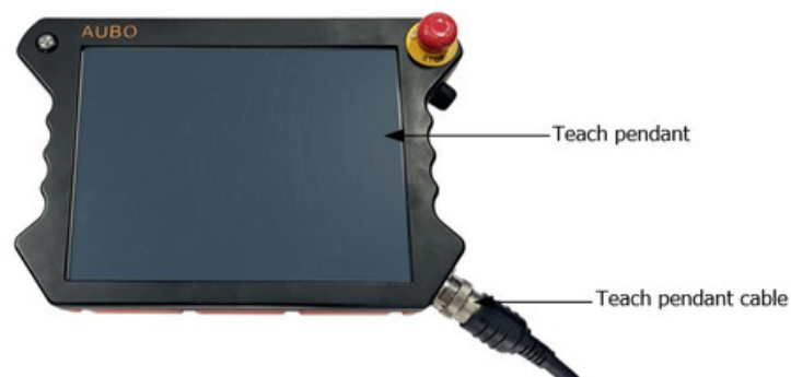
Figure 6-10 Teach pendant cable connected to the teach pendant
