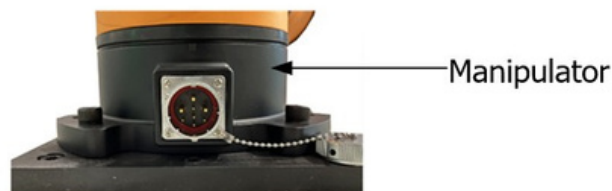
Figure 6-12 Manipulator cable connected to the Manipulator
