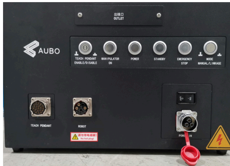
Figure 7-2 Front panel of the control box
