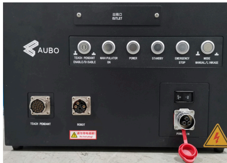
Figure 7-2 Front panel of the control box
